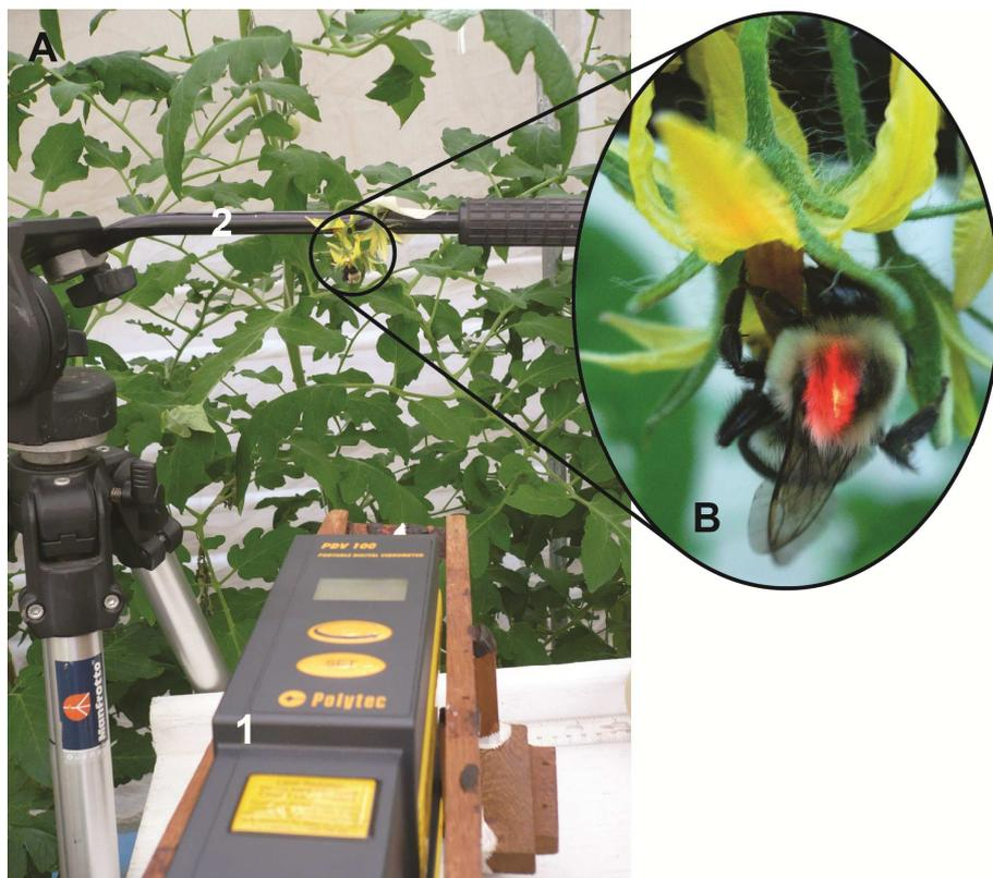
FIG. 2. Bumble bee (*Bombus impatiens*) vibration recording. (A) The setup showing the Laser Doppler Vibrometer mounted on a small four-wheeled cart (1) and the flower fixed to a tripod pan handle with adhesive tape (2) being visited by a forager. (B) The red dot on the scutum of the bee is the laser beam of the vibrometer.
